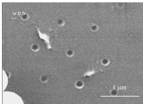
**Fig. 3** SEM image of nano-hole arrays formed on GST thin film surface after one pulse of KrF excimer laser irradiation at a laser fluence of 5.8 mJ/cm<sup>2</sup> and an incident angle of 0°.
