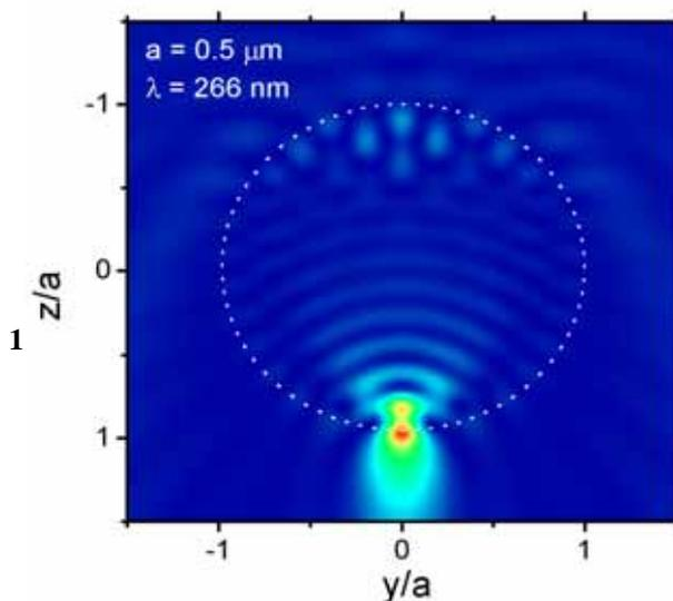
**Fig. 4** Laser light intensity  $|E|^2$  distribution inside & outside a 1.0 μm PS particle illuminated by a laser pulse at  $\lambda = 266 \text{ nm}$ .
