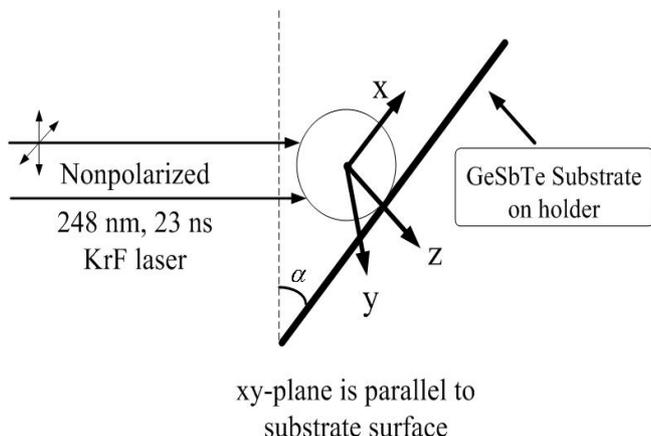
**Fig. 2** Schematic drawing of experiment setup for GST thin film surface nanopatterning.
