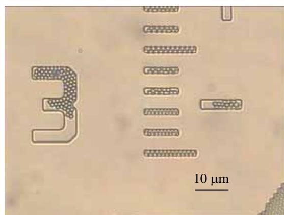
**Fig. 7** Optical images of transparent nanoparticles deposited inside pre-patterned structures by the self-assembly method.
