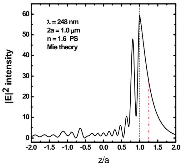
**Fig. 9** Laser light intensity along laser irradiation direction ( $z$ -axis,  $z = 1.0$  is the particle contacting point to the substrate.) during the KrF excimer laser irradiation of 1.0  $\mu\text{m}$  PS particle.
