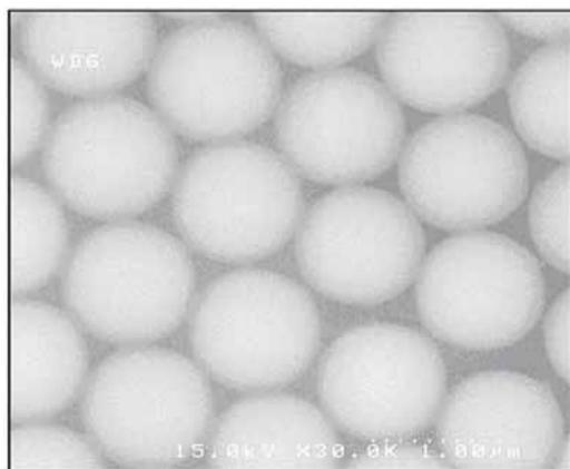
**Fig. 1** Optical image of 2D PS particle mask prepared by self-assembly on a 100-nm GST/Al thin film surface.
