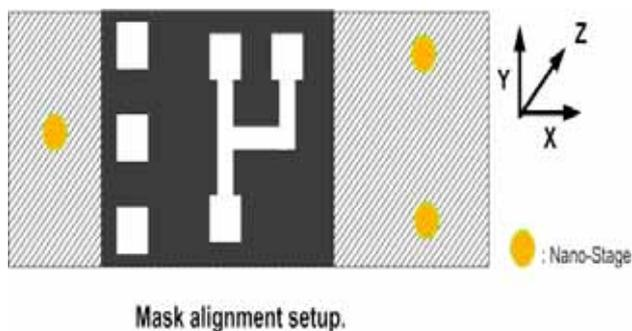
**Fig. 10** Mask alignment and three sets of ellipsometers (yellow circle points) to ensure the mask parallel to the substrate with a same distance in dozens of nanometers for the light enhancement.
