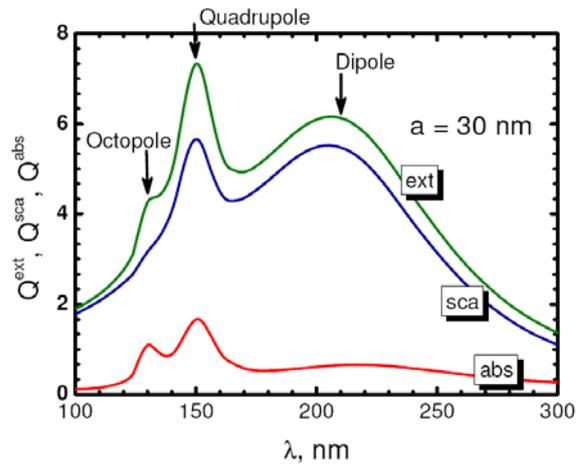
Fig. 2. Inverse hierarchy of resonances for an aluminum particle in vacuum. Normalized extinction, scattering and absorption cross-sections,  $Q^i = \sigma^i / \pi a^2$ , for a particle with  $a = 30$  nm as functions of incident light wavelength  $\lambda$ . Points of dipole, quadrupole and octopole resonances are indicated with arrows. The extinction cross-section of the quadrupole resonance is the greatest. With  $a = 40$  nm the octopole resonance becomes the greatest [11].
